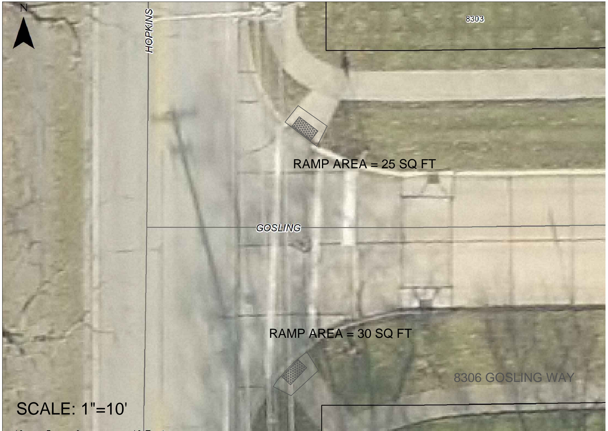
RAMP REPLACEMENT AT HOPKINS RD. & GOSLING WAY
