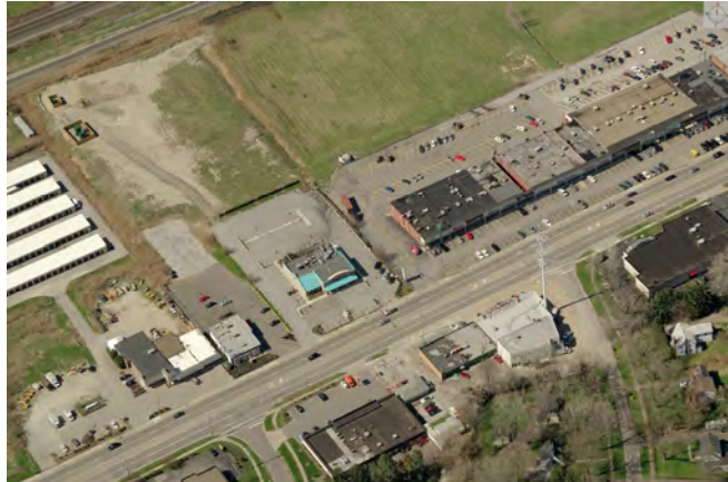
Figure 5.3 Redundant driveways along US 20 add points of conflict that make traffic patterns unpredictable, increase the risk of accidents, and contribute to traffic delays.
