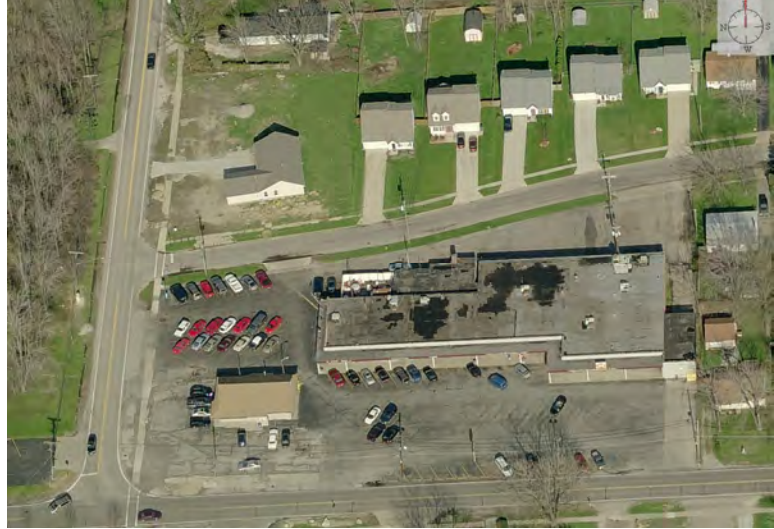
Figure 5.2 Continuous curb cuts are unattractive and unsafe, and make it difficult to tell where a road ends and a parking area begins.
