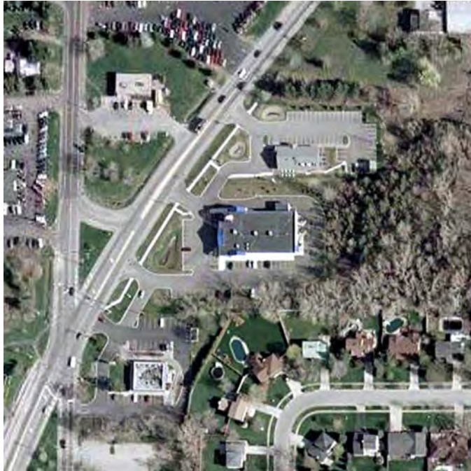
Figure 5.4 Cross-access driveways connect the parking areas of three separate businesses in Amherst, New York.
